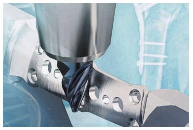
According to Inovatools, Curvemax curve segment mills can machine a titanium bone plate up to 85 % faster than conventional ball-shaped mills.
