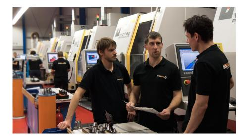
Modern grinding technology, operated by expert specialists, forms the basis for high-quality tool manufacturing.
